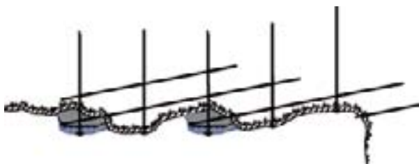
Fig 7.06 Sprayed rib, thickness 150-250 mm, radial bolts and spiling before the next blast.
