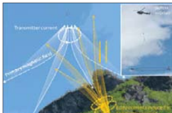
Figure 53: Fundamentals of AEM: A helicopter towed frame containing a wire loop acts as a strong EM transmitter with currents of up to 100 A (63 kAm 2 N/A). This primary magnetic field induces electrical eddy currents in conductive ground. These eddy currents in turn induce a secondary magnetic field which is being picked up by receiver coils on the same towed frame. The exact quantity and frequency content of the received signals contains information about the conductivity structure of the subsurface, which finally needs to be extracted from the data via sophisticated inversion algorithms.
