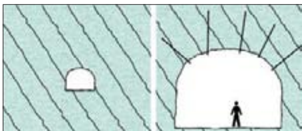
Figure 5. Example on the importance of the size of the cross section of the underground opening as related to the stability.
