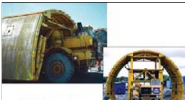
Figure 20. Example of formwork installed on a dumper; (picture from the Frøya tunnel)
