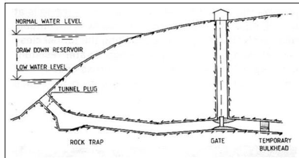
Figure 3.4. Principle of lake tap (Buen 1988)
