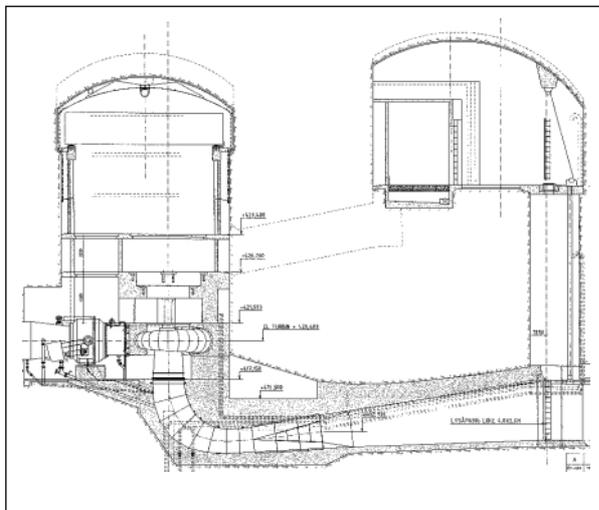
Figure 3.1. Cross section of a Norwegian power plant
