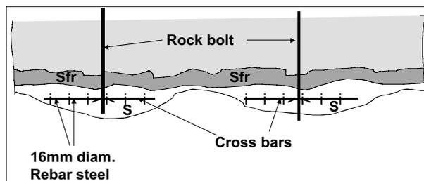
Figure 6.2. Principal sketch of two reinforced ribs of sprayed concrete with one layer of reinforcement (Grimstad et al 2002)
