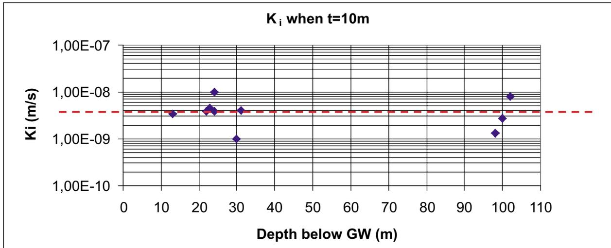
Figure 9.3. Hydraulic conductivity in the grouted zone from recent tunnel projects.
