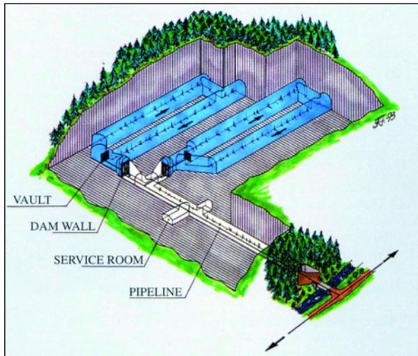
Figure 3.9. The Høgåsen underground water tank in Trondheim. Commissioned 1993. Capacity: 22 000m<sup>3</sup>
