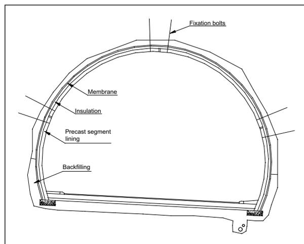
Figure 10.1. Pre-cast concrete segment lining
