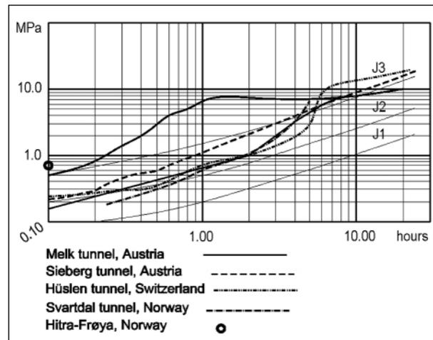
Figure 6.5. Examples of strength developments using 7% Meyco SA 160
