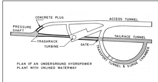
Figure 3.3. Plan of an underground hydropower plant (Broch 1985) Lake tap
