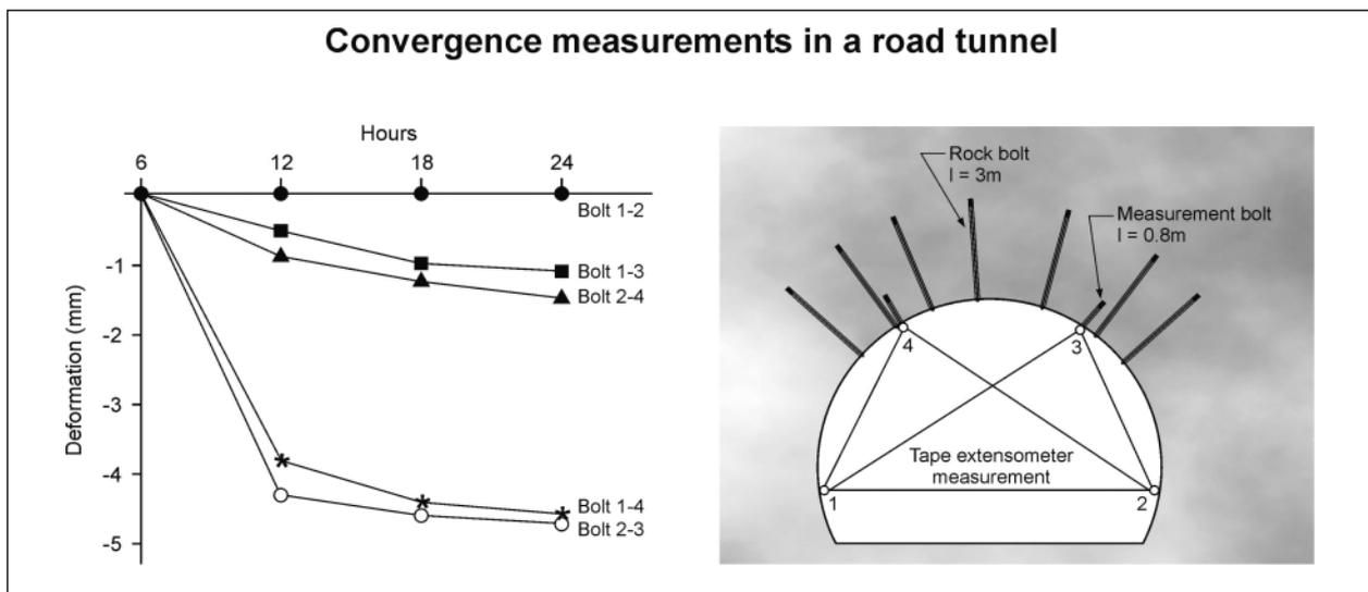
Figure 4.5. Convergence measurements in a tunnel
