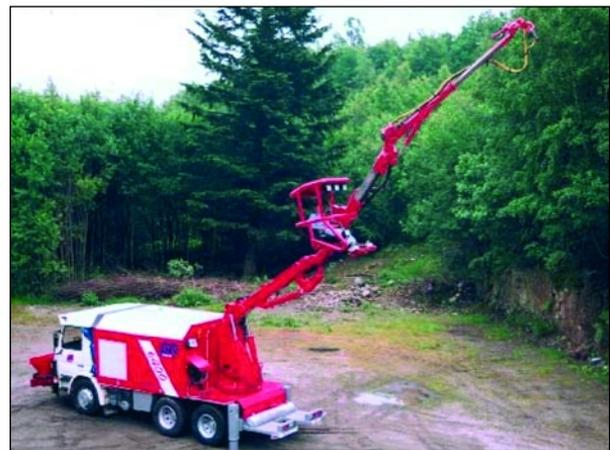
Figure 7.2. Sprayed concrete robot
