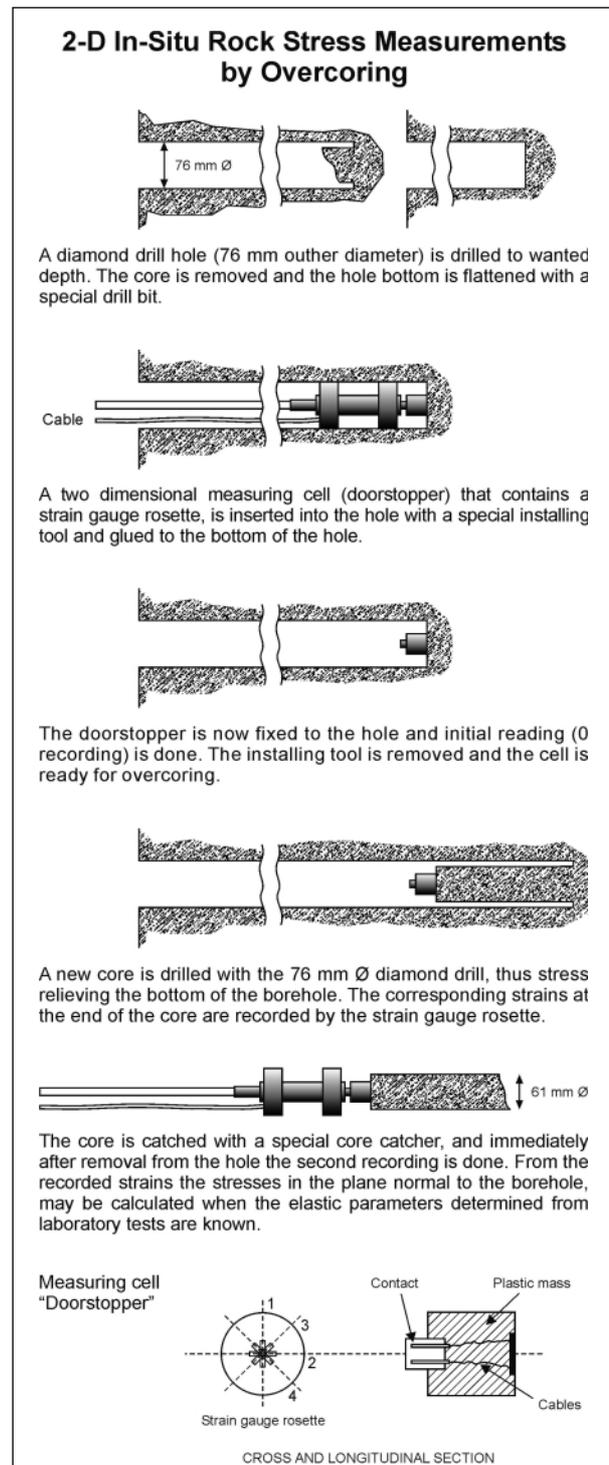
Figure 4.1. Principle for 2-D ("Doorstopper") overcoring method for rock stress measurement
