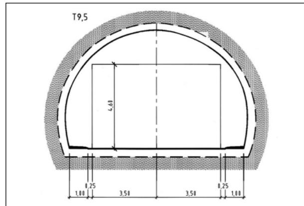
Figure 3.6. Cross section of a typical Norwegian road tunnel
