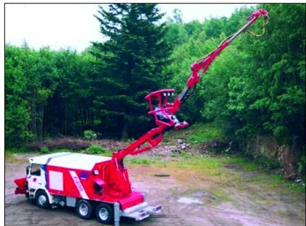
Figure 7.2. Sprayed concrete robot
