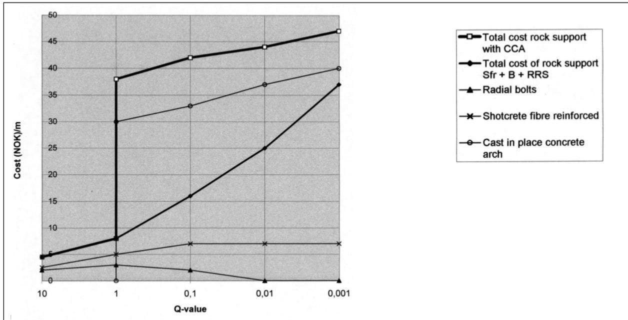
Figure 6.4. Cost comparison of applicable methods
