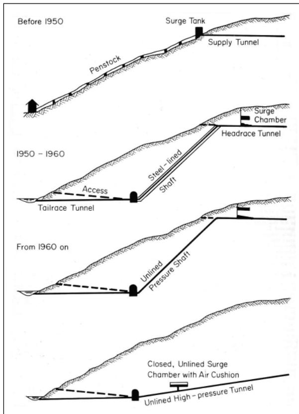
Figure 3.2. The development of the general layout of hydropower plants in Norway (from Broch 1985)
