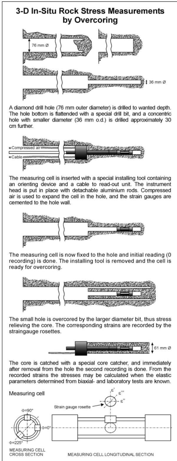
Figure 4.2. Principle 3-D overcoring method for in-situ rock stress measurement
