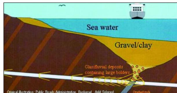
Figure 6.6. Ground freezing in the Oslofjord tunnel
