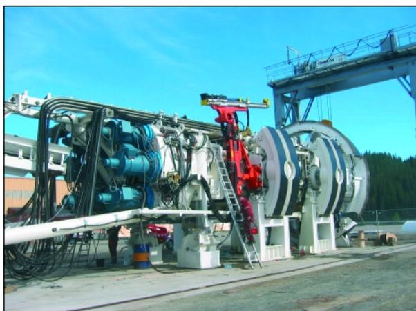
Figure 8.1. Open hard rock TBM
