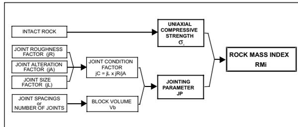
Figure 5.2. The input parameters to RMI (from Palmström, 1996)
