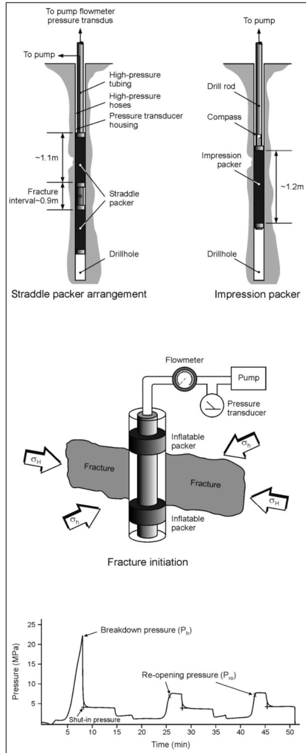
Figure 4.3. Principle for hydraulic fracturing
