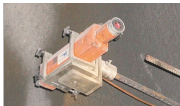
LASER FOR DIRECTION CONTROL.
