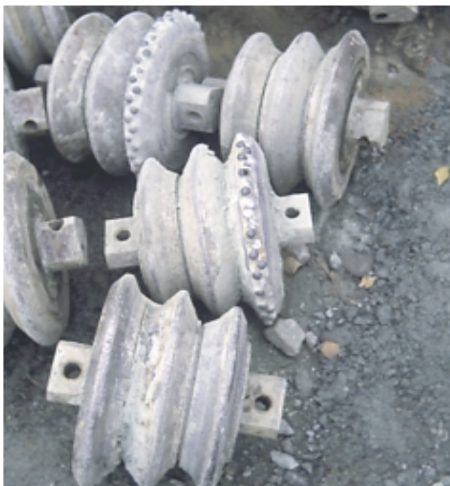
Fig. 1. Triple ring cutters, some with tungsten carbide inserts.
