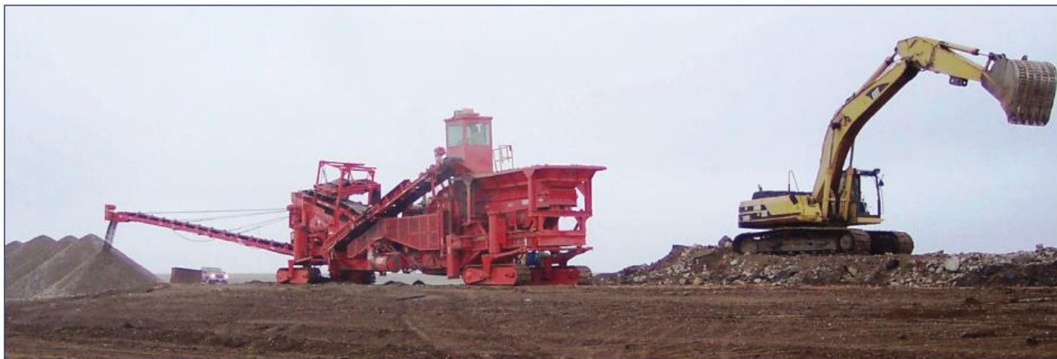
Figure 4. Paradigm in-place concrete recycling equipment in operation in Oklahoma (photo courtesy of Duit Construction)
