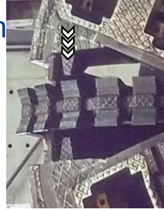
Wear Protection on the cutter head
