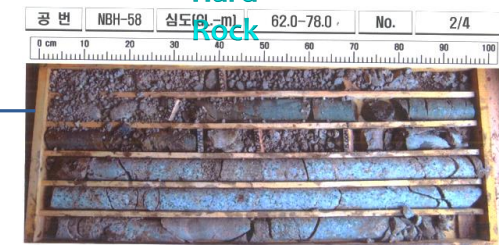
Weathered Rock/Fracture Zone
