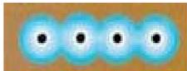
Closure of frozen earth wall
