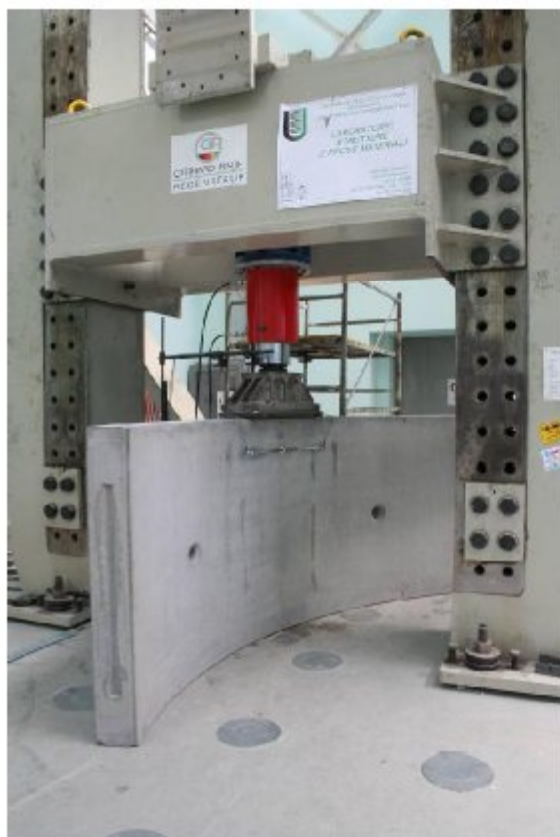
Fig. 6 – Point load test set up
