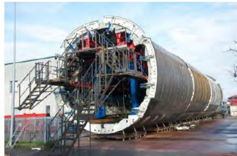
Secondary Lining Shutters Under Construction
