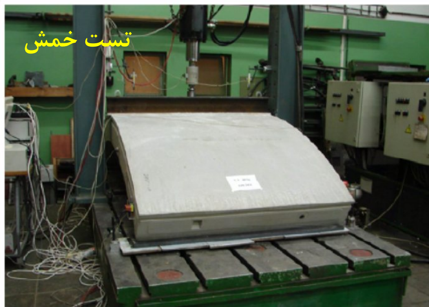
FIGURE 7. Segment bending (left: segment installed in the test machine; right: a detail of the fractured surface).
