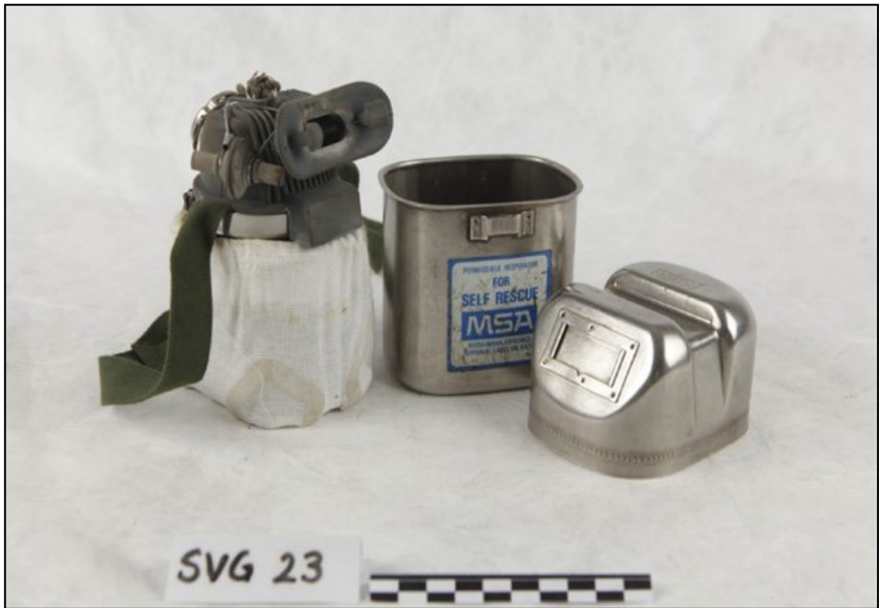
Figure 4: Picture of a self-saver; each worker in tunnel shall have this available
