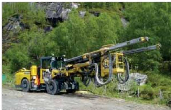
Figure 3. Small size 2-boom tunnel machines
