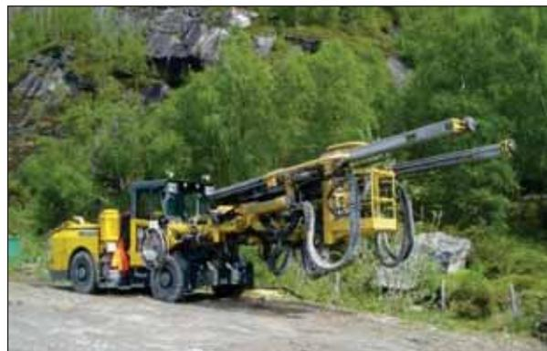
Figure 3. Small size 2-boom tunnel machines
