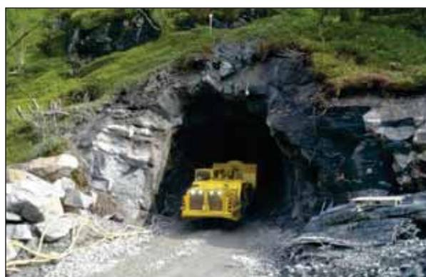
Figure 4. Low height mucking and transport equipment
