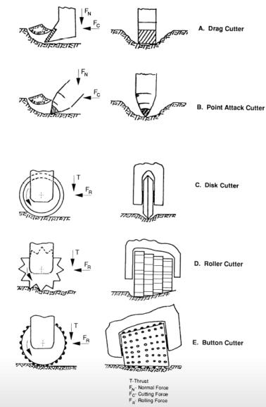
Fig. 22.1.1. Rock cutting techniques (after Roxborough and Rispin, 1973).
